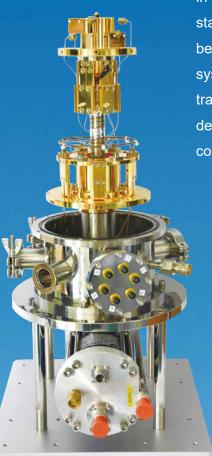
The ultra-low temperature cryostat (Limit temperature < 2.3K) used in superconducting single photon detection system(SNSPD) is a standard and technically mature product of our company, which has been applied in quantum communication successfully. The SNSPD system using this cryostat has an apparent advantage over traditional semiconductor (APD, PMT) detection technology in detection performance (Including detection efficiency and dark count, etc.).
